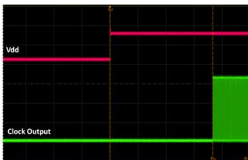
Figure 17. Startup Waveform vs. Vdd
